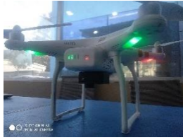
Fig. 2. Experimental Setup (Agrocam attached with Phantom 3 drone).
